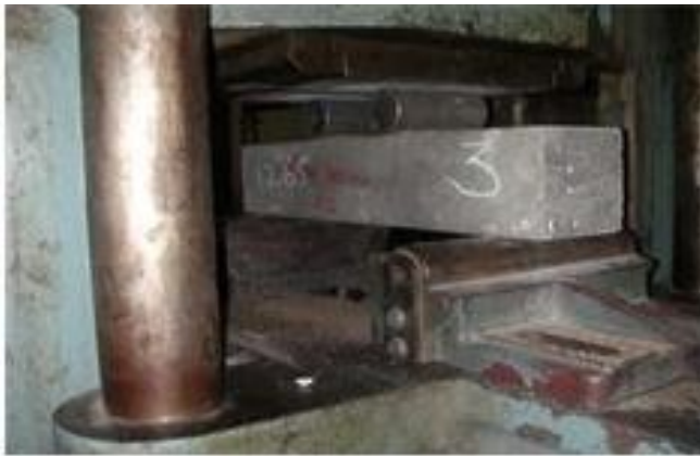
Fig No. 12 Test for flexural strength of Concrete
