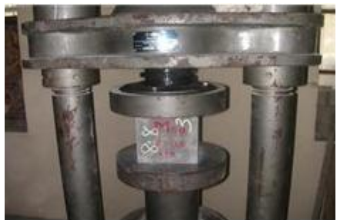
Fig No. 11 Test for Compressive strength of Concrete
