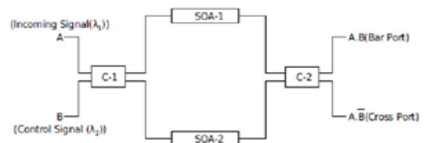
Fig. 2. SOA based Mach-Zehnder Interferometer switch [8]
