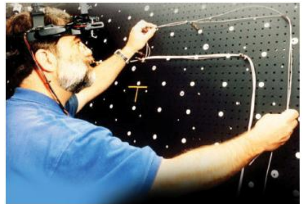
Researchers at Boeing used a see-through HMD to guide the assembly of wire bundles for aircraft. Courtesy of David Mizell.
