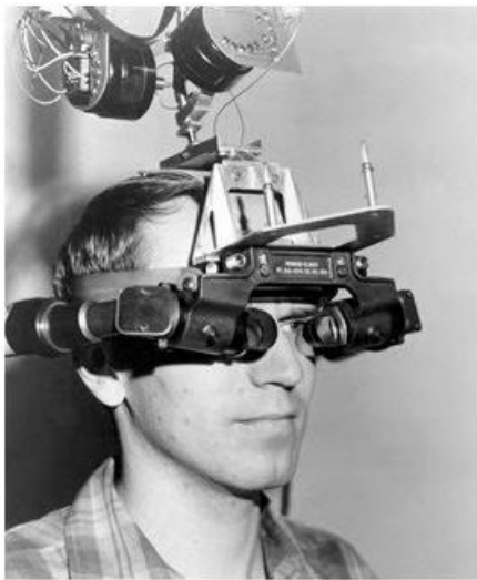
Figure 1.2 The Sword of Damocles was the nickname of the world's first head-mounted display, built in 1968. Courtesy of Ivan Sutherland.
