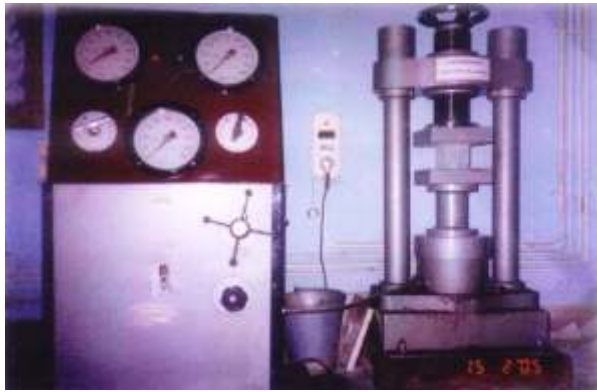
Compressive Strength Test on Cube
