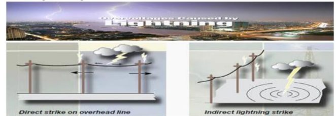
Fig (2)-Over Voltages Due To Lightning
