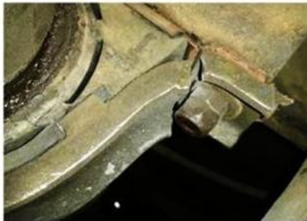
Fig.9 crack at the fillet region in working condition
