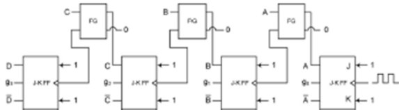
Fig. 5. Proposed design of 4-bit reversible sequence counter.
