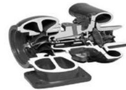
Fig 6: Turbocharger cut-away highlighting the twin-entry volute geometry, allowing differently pulsed exhaust gases to remain separate [35]
