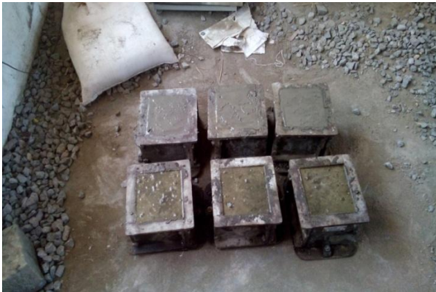
Figure –3.1 Casting of Specimens
