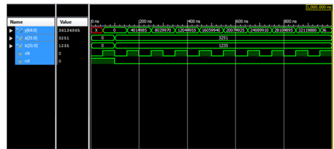
Fig.19: Simulation of 32bit-MAC using 32x32 vedic multiplier with DKG Logic gate
