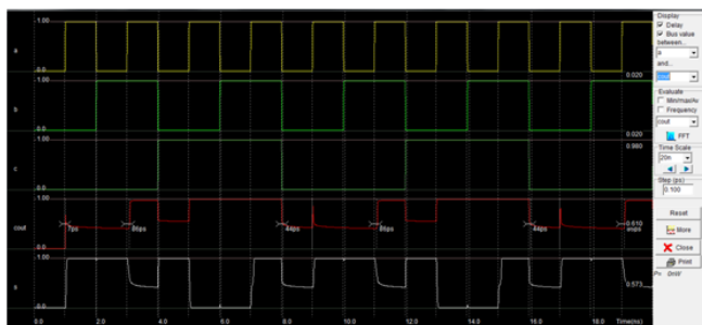
Fig 7: Layout Simulation of single gate MOSFET full adder
