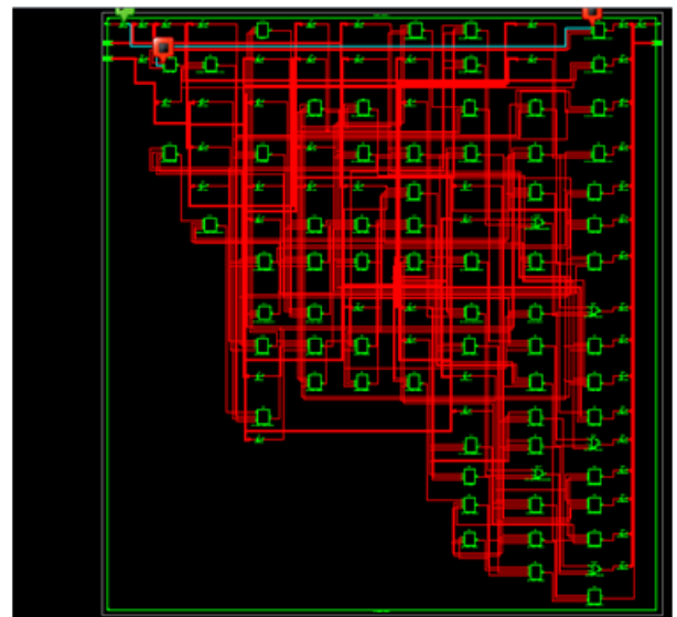
Fig.9: Technology Schematic of 16bit-BK-BEC Carry select adder
