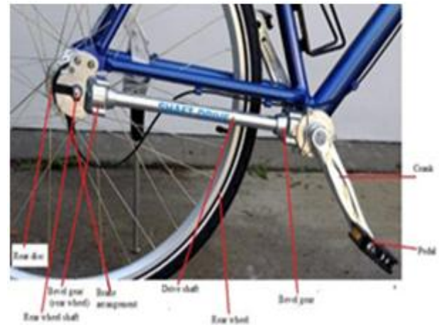
Fig4. components of shaft driven bicycle
