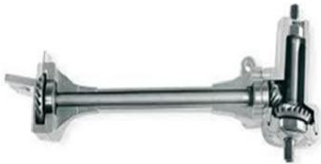
Fig2. Shaft drive for bicycle
