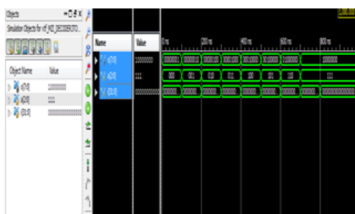
Fig.16.d: Simulation of All-Optical realization of the reversible 3to8 Decoder
