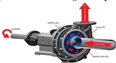
Fig: 1.2 cut section of impeller and parts of pump
