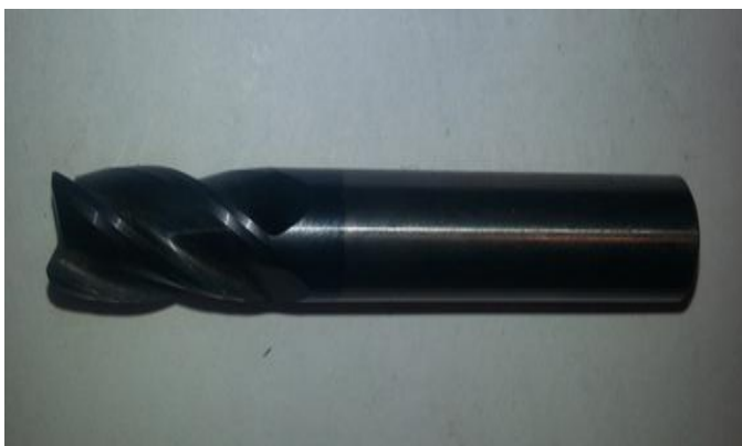
Fig 6.3 Failed milling cutter
