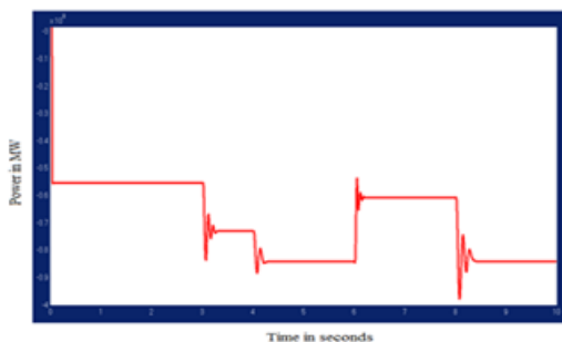
Fig 13: Real Power Flow Control in transmission line using TCSC with FLC from area2 to area1
