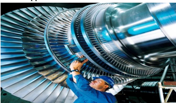
A rotor of a modern steam turbine, used in a power plant
