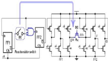
**Fig 3: Schematic of proposed E-TSPC based divide-by-2/3 prescaler.**
