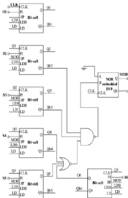
**Fig 5: Asynchronous 6-Bit S-Counter.**
