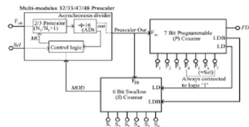
**Fig 1: Proposed dynamic logic multiband flexible Divider.**
