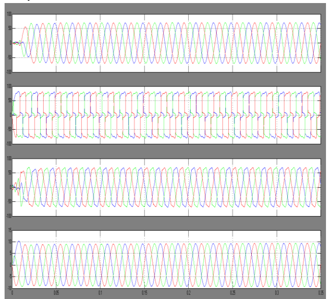
Fig.14 Simulation results for Balanced Non Linear Load (a) Source current. (b) Load current. (c) Compensator Current. (d) Wind Generator (Induction Generator) Current.
