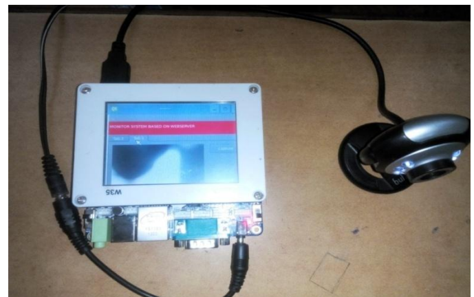
Figure 4: hardware device connection
