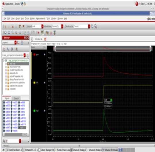
Figure 7 shows the voltage drop for mismatched inputs on proposed comparator.
