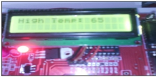
Fig 8: If the room temperature is increases the temperature sensor detected and the information display on the lcd screen like high temperature.
