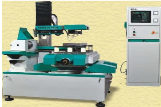
Figure 1.3: EZEECUT PLUS Wire cut EDM
