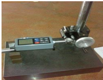
Figure 2.3: Surface Roughness Tester TR-200 Used for the
