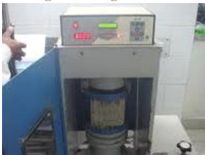
Fig. Tests for compressive strength of concrete
