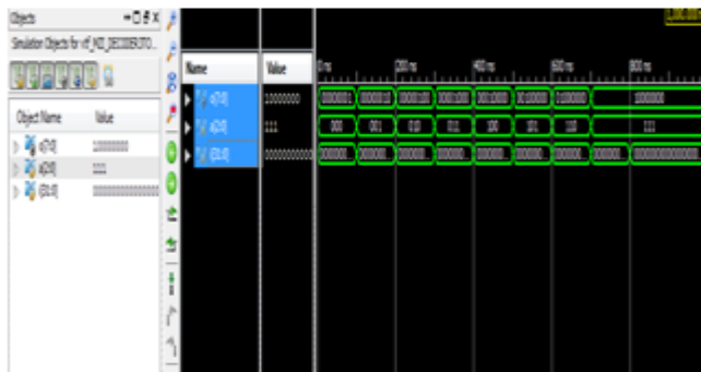
Fig.16.d: Simulation of All-Optical realization of the reversible 3to8 Decoder
