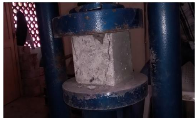
Fig 2: compressive strength for RAC
