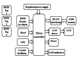
From the above figure, we can see that the device which is able to perform the task is a LPC 2148 Micro controller. There is RFID reader send data to micro controller then the buzzer indicates alerts and send message through GSM to the predefined numbers, LPC 2148 Micro Controller is programmed using embedded C programming language.
