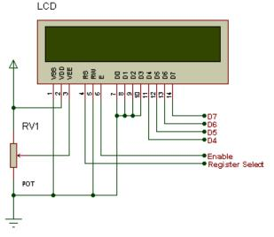
The LCD requires 3 control lines as well as either 4 or 8 I/O lines for the data bus. The user may select whether the LCD is to operate with a 4-bit data bus or an 8-bit data bus. If a 4-bit data bus is used the LCD will require a total of 7 data lines (3 control lines plus the 4 lines for the data bus). If an 8-bit data bus is used the LCD will require a total of 11 data lines (3 control lines plus the 8 lines for the data bus).
