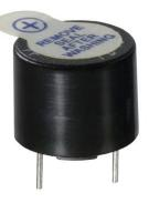
Basically, the sound source of a piezoelectric sound component is a piezoelectric diaphragm. A piezoelectric diaphragm consists of a piezoelectric ceramic plate which has electrodes on both sides and a metal plate (brass or stainless steel, etc.). A piezoelectric ceramic plate is attached to a metal plate with adhesives. Applying D.C. voltage between electrodes of a piezoelectric diaphragm causes mechanical distortion due to the piezoelectric effect.
