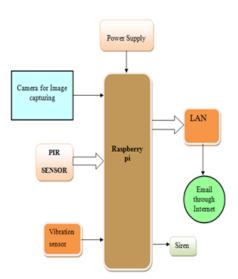
The **Raspberry Pi** is a credit-card-sized single-boar computer developed in the UK by the Raspberry Pi Foundation. The Raspberry Pi has a Broadcom BCM2836/2837 system on a chip. It does not include a built-in hard disk or solid-state drive, but Uses an SD card for booting and long-term storage.
