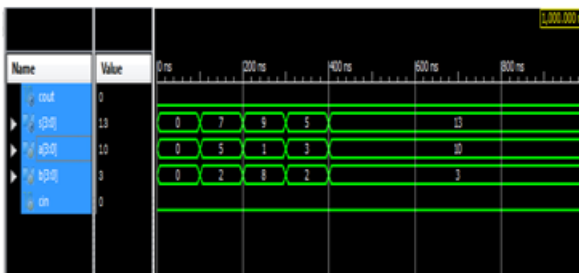
Figure 14: simulated outputs for proposed reversible 4bit adder
