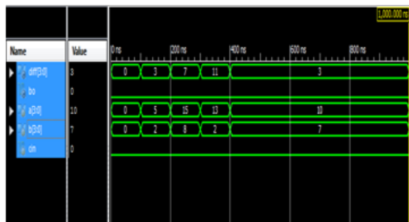
Figure 15: simulated outputs for proposed reversible 4bit subtractor
