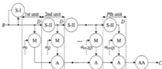
Fig. 3. Cut-set retiming of PSFG of finite field RB multiplication over (GF(2 m )) Where "D" denotes delay.
