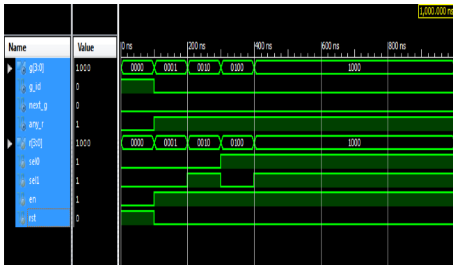
Fig10: Simulation output waveform of an Index-based Round Robin (IRR) arbiter.
