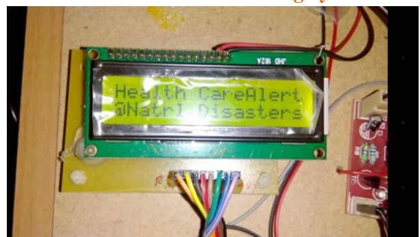
At- Home Health Monitoring System Result on LCD
