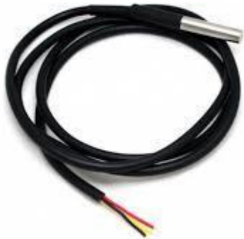
Fig: Temperature sensor
