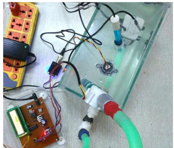
Fig: System design model of water quality monitoring system using IOT
