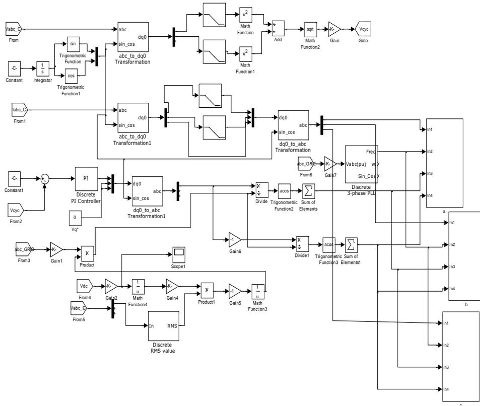
Figure 8: Receiving end side controller
