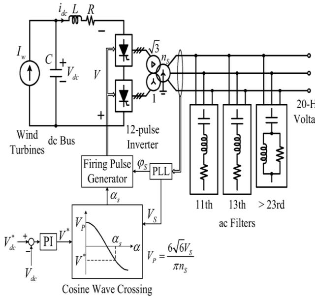
Figure 2: Sending-end inverter control.
