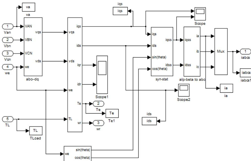
Figure 10: Induction motor modeling
