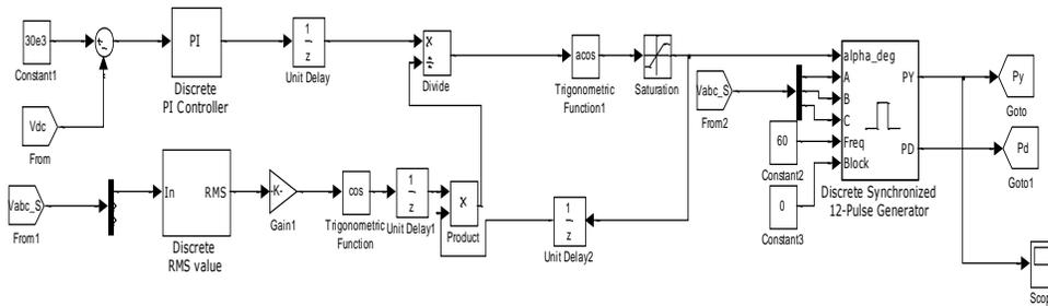
Figure 7: Sending end side controller:
