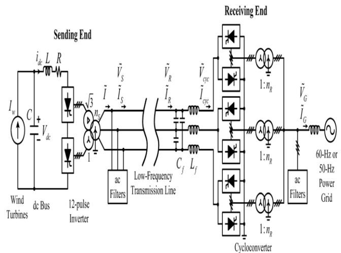
Figure 1: Configuration of the proposed LFAC transmission system
