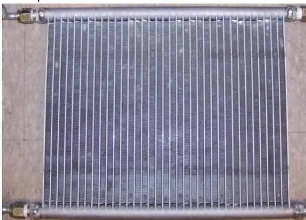
This heat exchanger allowed connections on either side of both headers. The heat exchanger was connected to the system in two ways: with the inlet and outlet on the opposite side and inlet and outlet on the same side. Figures 2.3 and 2.4 illustrate this in greater detail. The location of pressure measurements is also shown, with the pressure transducers represented as circles. The values that are boxed indicate pressures calculated by the model.
