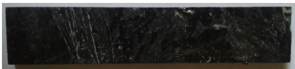
Fig 9: Specimen of ASTM D618 (No 5)
