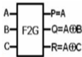
Fig.4 Block diagram of Feynman Double gate.
