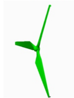
Fig.7 Wind Turbine (With Winglet 90°)
