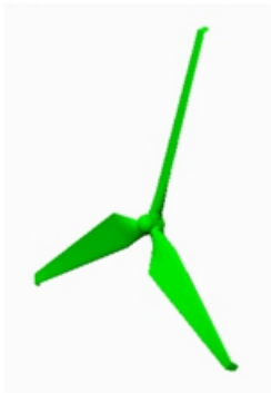
Fig.5 Wind Turbine (With Winglet 60°)
