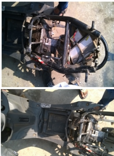
Fig.6.8 Space Allocation for batteries
