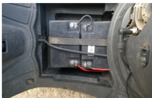
Fig .Arrangement of Batteries at Foot rest
