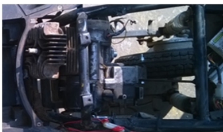
Fig.6.2 Arrangement of fuel engine to E-bike
