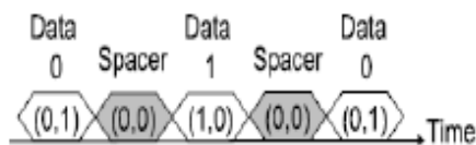
Fig. 3. Example of data transfer based on four-phase dual-rail protocol.
