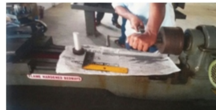
MAKING OF M.S. PARTICLES ON LATHE
