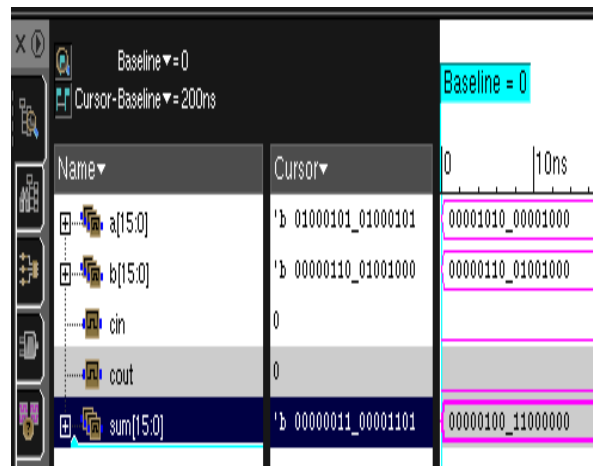
Fig11: Simulation Result of 16-bit Reversible kogge Stone Adder
