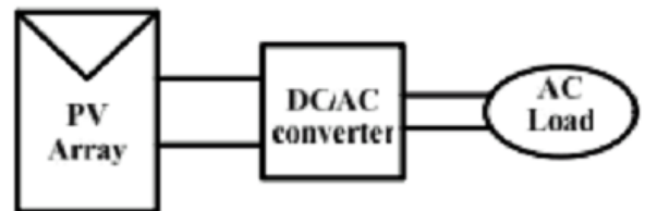
Fig.1. Block diagram representation of Photovoltaic system
