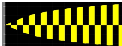
Fig 6 Three level inverter voltage
