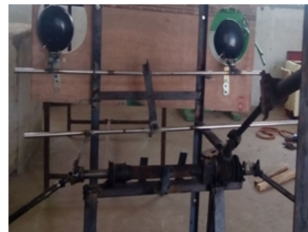
Fig : links attached to the steering mechanism and frame
