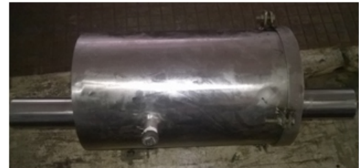
Fabricated Catalytic Converter Cartridge Recharged with Coal Stainless steel Filter Body Cap
