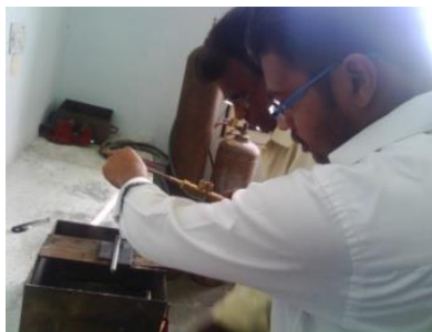
b. brazing work on rod
