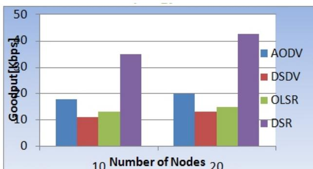
Figure: 9 Good put of Mesh topology
