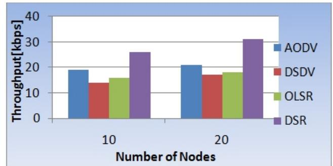
Figure: 10 Throughput of Mesh topology
