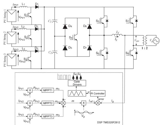
**Multistring Five-Level Inverter With Control Algorithm Implemented In Dsp Tms 320f2812.**
