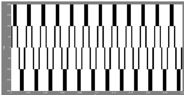
Fig.5.3.Simulated waveforms of phase voltage VAB of inverter stage [Scale:100 V/div]
