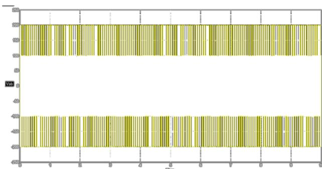
Fig.5.6.Simulated waveform of Five-level inverter topology of CCHB inverter
